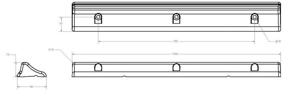
Fixings ;-  $3 \times M10 \times 120$ mm long Stainless Steel A2 grade coach screws with mud guard washers and  $14\emptyset$  nylon Rediplugs
